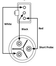
Ohm water Level Probe and Wiring Harness
