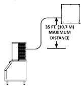
**35 ft. (10.7 m) Rise:** The maximum distance the Condenser or Condensing Unit can be above the ice machine.
